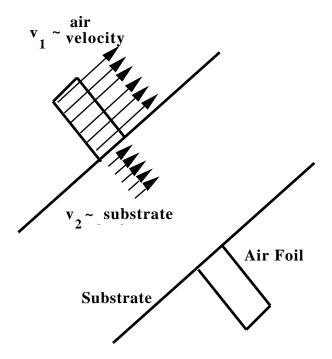
Figure 4. Kelvin-Helmholtz problem as it occurs in oven using air foils.
