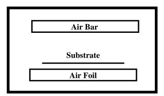
Figure 1. Oven configuration for edge mottle experiments.
